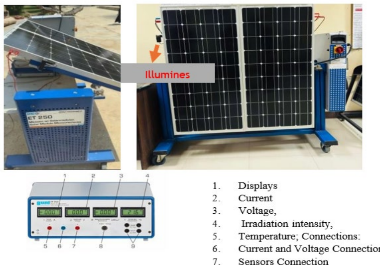
Fig.5 Solar Irradiance Measurement Setup
